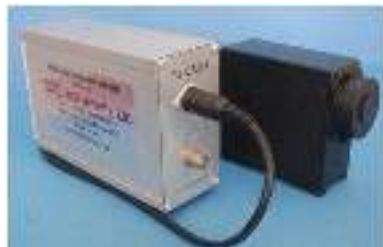
Golay cell example taken from QMC NEP \sim 200 \text{ pW}/\sqrt{\text{Hz}} (0.2 – 30THz)
