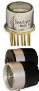
He-cooled bolometer example taken from QMC NEP \sim 3 \text{ pW}/\sqrt{\text{Hz}} (0.2 – 30 THz)
